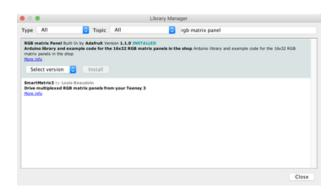
Now you are ready to test! Open up the IDE and load File $\rightarrow$ Examples $\rightarrow$ RGBmatrixPan el $\rightarrow$ testcolors\_16x32 (for the 16x32 panel) or File $\rightarrow$ Examples $\rightarrow$ RGBmatrixPanel $\rightarrow$ color wheel\_32x32 (for the 32x32 panel). There's also a testshapes\_32x64 example for boards with sufficient RAM.
