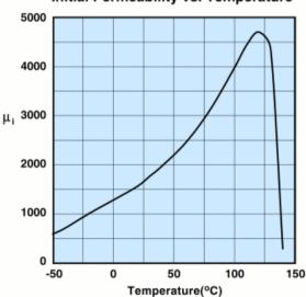
Measured on a 17/10/6mm toroid at 100kHz.
