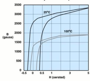
Measured on a 17/10/6mm toroid at 10kHz.
