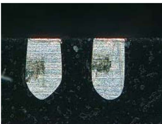
50 times insertion same IC
