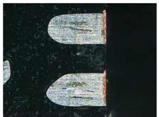
50 times insertion same IC
