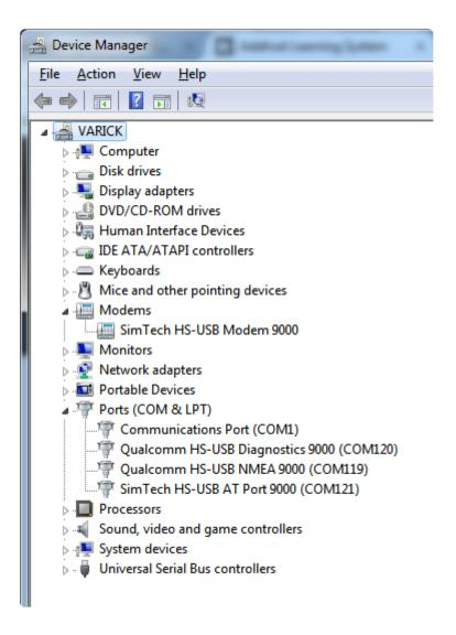
You can connect to the AT com port at any baud rate and send AT commands like normal. This makes it super easy to test out commands
