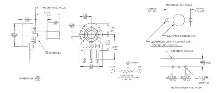
Series 270U Metal Shaft, Bushing Mount, Printed Circuit "U" Type Terminals
