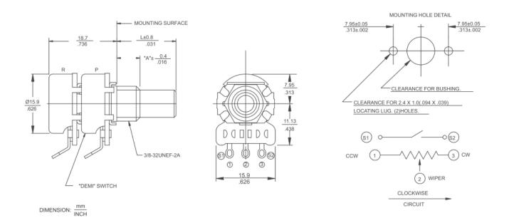
Series 270X-x-B Metal Shaft, Bushing Mount, Printed Circuit "X" Type Terminals, Rotary Switch
