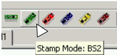
Click on the icon that corresponds to your BASIC Stamp model to automatically place the $STAMP directive in your program.
