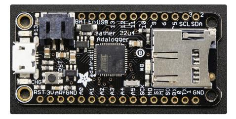
At the Feather 32u4's heart is at ATmega32u4 clocked at 8 MHz and at 3.3V logic, a chip setup we've had tons of experience with as it's the same as the Flora (https://adafru.it/dVI). This chip has 32K of flash and 2K of RAM, with built in USB so not only does it have a USB-to-Serial program & debug capability built in with no need for an FTDI-like chip, it can also act like a mouse, keyboard, USB MIDI device, etc.
