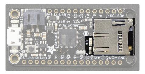
Since not all pins can be brought out to breakouts, due to the small size of the Feather, we use these to control the SD card!
