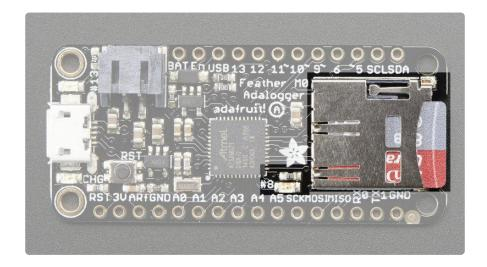
Since not all pins can be brought out to breakouts, due to the small size of the Feather, we use these to control the SD card!
