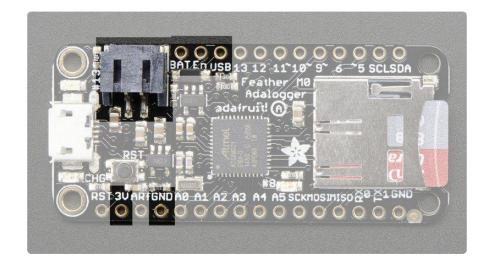
• GND - this is the common ground for all power and logic
