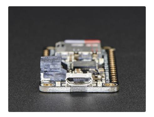
Comes fully assembled and tested, with a USB bootloader that lets you quickly use it with the Arduino IDE. We also toss in some header so you can solder it in and plug into a solderless breadboard. Lipoly battery, MicroSD card and USB cable not included (but we do have lots of options in the shop if you'd like!)
