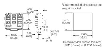
Hard mount sockets for relays with 4 poles Socket with printed circuit terminals is available for KUP relays, with 4 poles, with .110" (2.79mm) quick connect terminals. 27E043—with solder eyelet terminals. 27E419—with printed circuit terminals.
