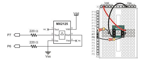
The program below, SimpleTilt.bs2, simply measures the pulse width, that is, the duration of tHx, for each axis. The raw values are displayed in the BASIC Stamp Editor's Debug Terminal. If you run the program, then tilt the accelerometer, you should see the values for each axis change.
