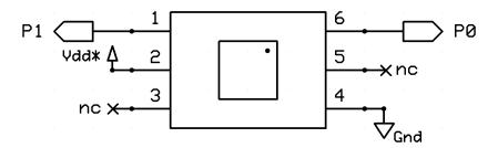
\*Vdd = 3.3V for Propeller Applications, 5V for BASIC Stamp Applications
