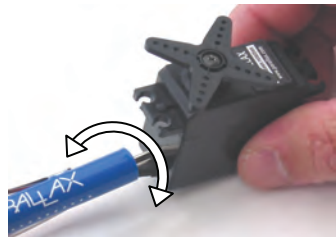
Figure 2-24 Center Adjusting a Servo
