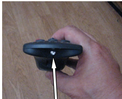
With a button pressed and held, the IR LED doesn't look any different.
