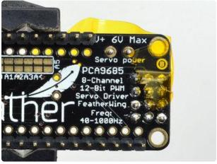
Solder in both pins of the terminal block. You can remove the tape when done.
