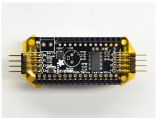
Again, use some tape to hold down the two header pieces in place to make soldering easier.
