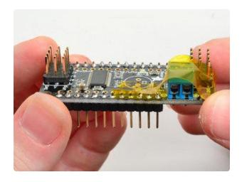
Last is the 3.5mm terminal block used for power. This is how you will provide the large amount of current that servos require.
