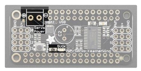
When the servo power pin is powered, the 5VOK LED will be lit. If this LED is not lit, the V+ pins will not have any voltage on them and the servos won't be powered.
