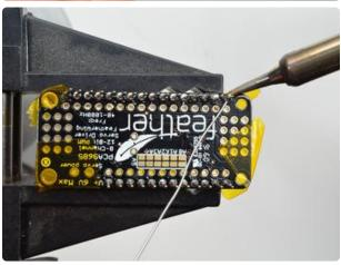
Next we will solder in the right angle header blocks used to plug in servos into the FeatherWing. There are two blocks, each are 3x4 headers in size.
