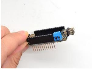
They go on either end. Make sure the long side of the headers is sticking off the top left & top right sides!
