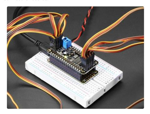
Since the FeatherWing only uses the I2C (SDA & SCL pins), it works with any and all Feathers- ATmega32u4, ATSAM M0 or ESP8266-based. You can stack it with any other FeatherWing or with itself (just make sure you have each wing with a unique I2C address) Check out our range of Feather boards here. (https://adafru.it/I7B)
