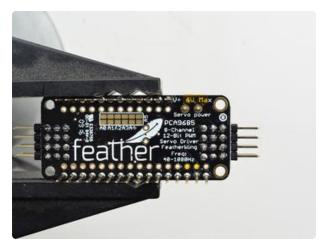
Solder in both pins of the terminal block.
