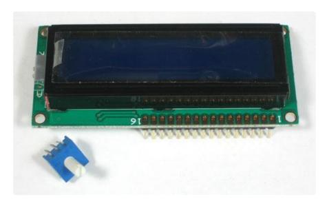
The easiest way we know of doing this is sticking the header into a breadboard and then sitting the LCD on top while soldering. this keeps it steady.
