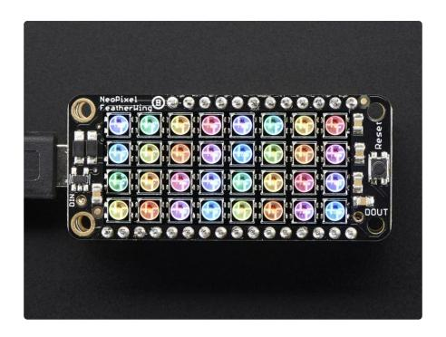
Put on your sunglasses before staring into these 32 configurable eye-blistering RGB LEDs. Arranged in a 4x8 matrix, each pixel is individually addressable. Only one pin is required to control all the LEDs. On the bottom we have jumpers for the DIN line to any of the I/O pins on a Feather. You can cut the default jumper trace and use any pin you like. (In particular, the default pin for Feather Huzzah ESP8266 must be moved, try pin #15!)
