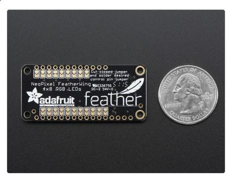
To make it easy to start, the LEDs are by default powered from either the USB power line or Battery power line, whichever is higher. Two Schottky diodes are used to switch between the two. This power arrangement is able to handle 1 Amp of constant
