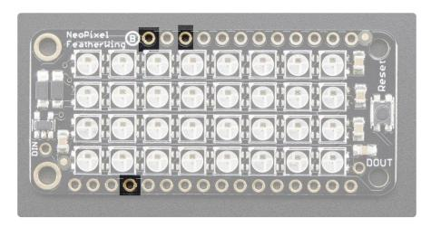
The bottom row's ground pin is also used of course, for both power and data ground reference.
