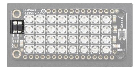
That means, if USB is plugged in, you'll get ~5V USB power. If the feather is running off of battery power, say a LiPoly battery, you'll get 3.7-4.2V power. While this is a little lower than spec, NeoPixels are only a little dimmer.
