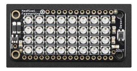
The NeoPixel FeatherWing is pretty easy to use, there's only one data pin (NeoPixels use a timing-based protocol to communicate). You also have 3 pins that can be used for power:
