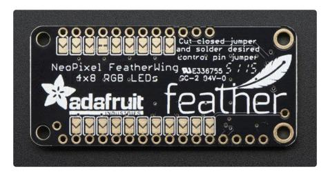
On the bottom, we have a range of pins that are available for use as the 'control pin'
