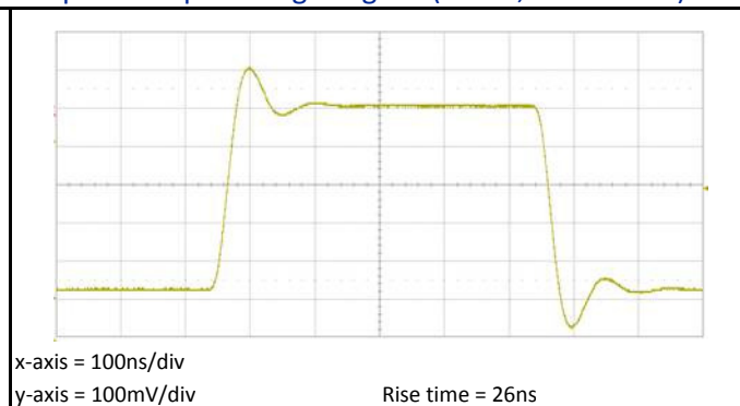
Response to pulsed light signal (M=25; \lambda = 860 nm)
