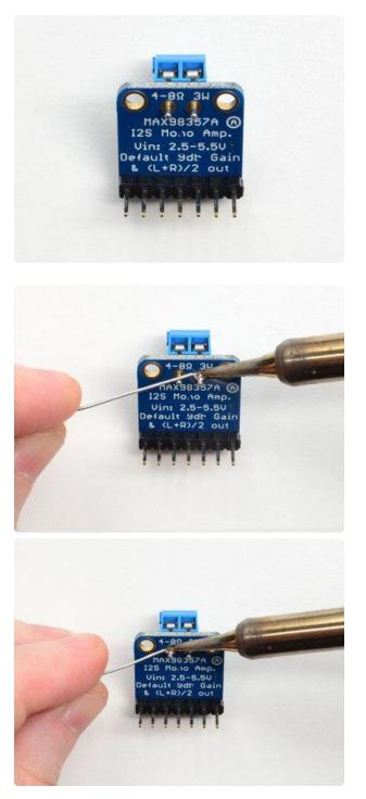
If you want to use a terminal block for connecting a speaker, place the 3.5mm terminal so the mouthes point out.
