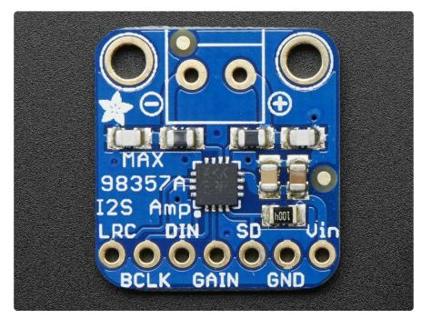
The MAX98357A is an I2S amplifier - it does not use analog inputs, it only has digital audio input support! Don't confuse I2S with I2C, I2S is a sound protocol whereas I2C is for small amounts of data.
