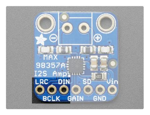
Three pins are used to receive audio data. These can be 3.3-5V logic
