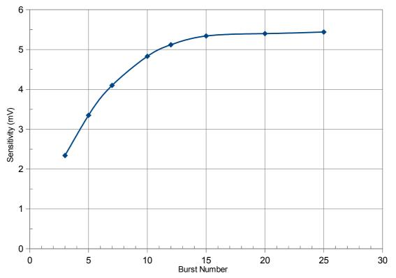
6 Bandwidth vs. Driving Burst Number: Driving voltage 10Vp-p square wave, Reflection target distance: 10cm
