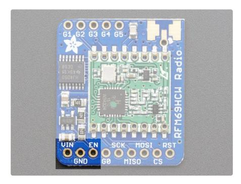
The left-most pins are used for power
