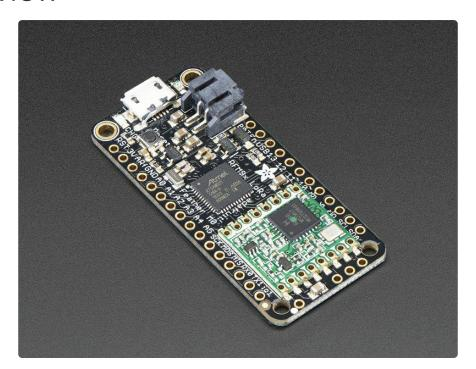
This is the Adafruit Feather M0 RFM95 LoRa Radio (433 or 900 MHz) - our take on an microcontroller with a "Long Range (LoRa) (https://adafru.it/mFZ)" packet radio transceiver with built in USB and battery charging. Its an Adafruit Feather M0 with a Long Range radio module cooked in! Great for making wireless networks that are more flexible than Bluetooth LE and without the high power requirements of WiFi. We have other boards in the Feather family, check'em out here (https://adafru.it/I7B).
