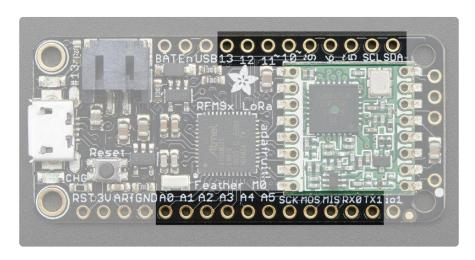
This is the general purpose I/O pin set for the microcontroller.
