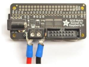
Plug the red wire into the + side, and the black wire into the - side.
