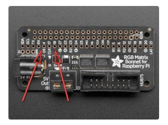
The "quality" option comes at a cost. First, you need to solder a jumper wire between GPIO4 and GPIO18 on the Bonnet or Hat board. Also, the normal sound output of the Raspberry Pi must be disabled. You can still use a USB sound adapter if needed, but audio over HDMI or from the 1/8" jack will not be present.
