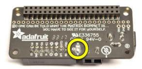
If you're using a 64x64 RGB matrix and either a Bonnet or a Rev C HAT, use your soldering iron to melt a blob of solder on the bottom solder jumper so the middle pad is 'shorted' to 8. (This is compatible with 64x64 matrices in the Adafruit store. For 64x64 matrices from other sources, you might need to use 16 instead, check the datasheet.)
