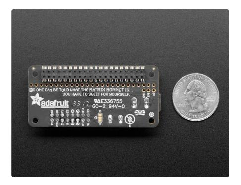
Works with any of our <u>16x32</u>, <u>32x32</u> or <u>32x64</u> RGB LED Matrices with HUB75 connections (https://adafru.it/emd). You can also <u>use 64x64 matrices by soldering a</u> <u>small jumper on the PCB</u> (https://adafru.it/BhY). Want more lights? No problem, chain multiple matrices together for a longer display - we've only tested up to 32x128 but it works just fine. The bigger the display the harder it is on the Pi, so keep that in mind if you're using a lower-powered Pi Zero.
