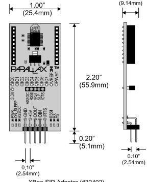
XBee SIP Adapter (#32402)
