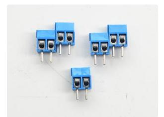
Next we will solder in the five 3.5mm terminal blocks used to connect power & the motors to the FeatherWing board.
