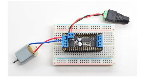
You must also supply 5-12VDC to power the motor. You can power the Wing via a connected DC Barrel Jack as seen above. A battery pack is good for portable use. Note that this will not power the Feather, that's normal - you want to keep separate power supplies and the Feather is best powered by a separate lipoly battery
