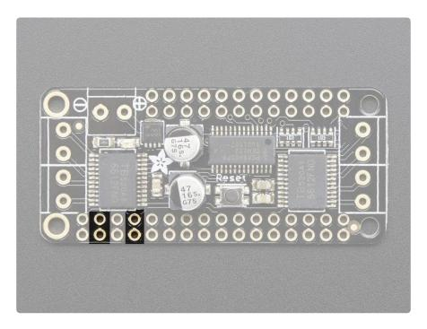
The logic power to the I2C expander and motor pins comes from the Feather's 3.3V regulator, 3.3V and ground are both required.
