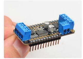
The terminal blocks have interlocking dovetailed grooves on the sides. Line two of them up as shown, and press down to lock them together as a 4position terminal block. It is a snug fit, so you may have to press hard.
