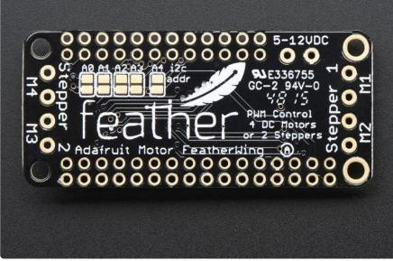
There are two motor sets. The left set is known as Stepper 1 or M1 + M2. The right set is Stepper 2 or M3 + M4
