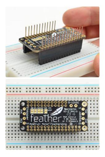
Flip it upside down so that the stacking headers fit over the headers in the breadboard
