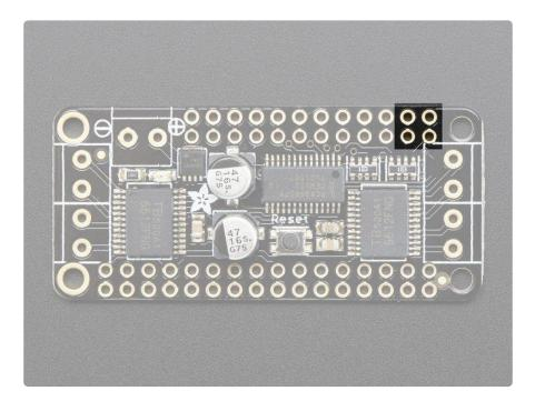
All data and control is done over I2C so it works with any and all Feathers! No need to set any PWMs. SDA and SCL are highlighted above. There are 10K pullups to 3.3V on each.
