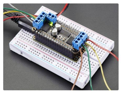
A Feather board without ambition is a Feather board without FeatherWings! This is the DC Motor + Stepper FeatherWing which will let you use 2 x bi-polar stepper motors or 4 x brushed DC motorx (or 1 stepper and 2 DC motors). Using our <u>Feather</u> <u>Stacking Headers</u> (http://adafru.it/2830) or <u>Feather Female Headers</u> (http://adafru.it/ 2886) you can connect a FeatherWing on top or bottom of your Feather board and let the board take flight!
