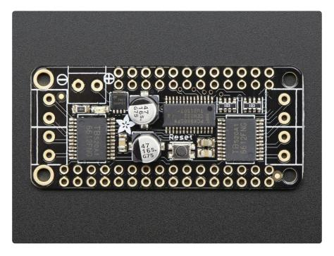
The original Adafruit Motorshield Kit (http://adafru.it/1438) is one of our most beloved shields, which is why we decided to squish it all together on a FeatherWing to make something even smaller, lighter, and more portable! Instead of using a latch and the Arduino's PWM pins, we have a fully-dedicated PWM driver chip onboard. This chip handles all the motor and speed controls over I2C.
