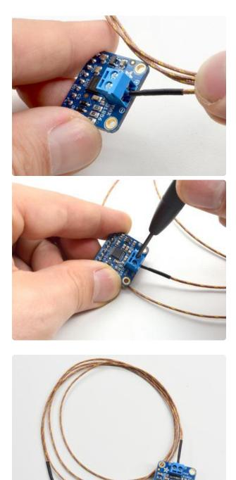
Insert the thermocouple wires and tighten down the clamps with a small Phillips or flat screwdriver
