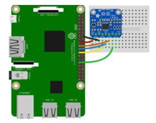
Here's the Raspberry Pi wired with SPI:
