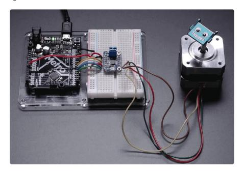
There's two digital inputs per H-bridge (one for each half of the bridge), you can PWM one of the inputs to control motor speed. Runs at 2.7V-10.8V logic/motor power. The motor voltage is the same as the logic voltage, but logic voltage from 2.7V or greater will work so no need to worry if you are powering the motors from 9V and using 3.3V logic. For higher voltages, check out the TB6612. (https://adafru.it/sdc) For much higher voltages and currents check out the DRV8871! (http://adafru.it/3190)
