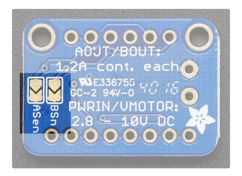
If you want a lower current limit, remove/destroy the  $0.2\Omega$  resistor on the board and add your own resistor value between Asen or Bsen and ground.
