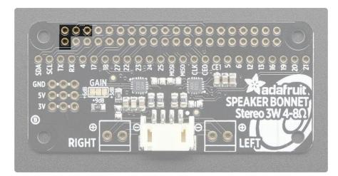
The two amplifier chips use the 3V + 5V + GND power pin at the 'top' of the 2x20 header. If using 3W speakers, you can draw a significant amount of current, over 1.5 Amps! Make sure you power your Pi with a good wall adapter like our 2.4A microUSB power plug.
