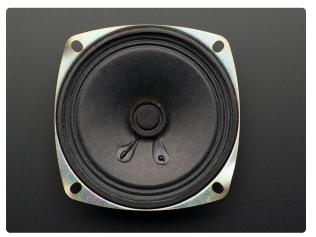
Speaker - 3" Diameter - 8 Ohm 1 Watt Listen up! This 3" diameter speaker cone is the perfect addition to any audio project where you need an 8 ohm impedance and 1W or less of power. We particularly like this cone as... https://www.adafruit.com/product/1313 You can also use other 'audio' devices like sonic transducers! These are devices you can put down onto a surface like a table, to make it into a speaker.
