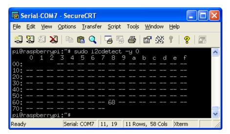
Once you have the Kernel driver running, i2cdetect will skip over 0x68 and display UU instead, this means its working!
