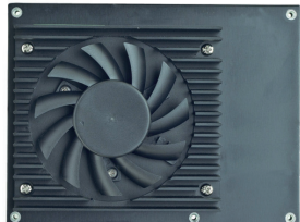
// Image 3: Build a Cooling Solution: Active Uni cooler mounted onto regular heatspreader
