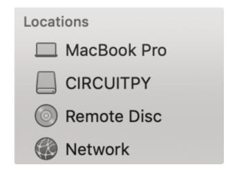
After it finished uploading, and with the Circuit Playground board connected over USB, it should appear on your computer as a flash drive called CIRCUITPY.
