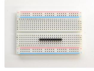
Prepare the header strip: Cut the strip to length if necessary. It will
