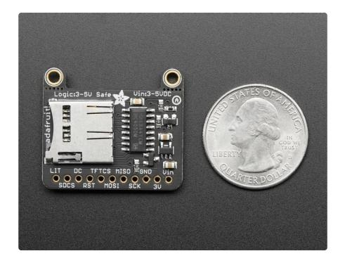
The breakout has the TFT display soldered on (it uses a delicate flex-circuit connector) as well as a ultra-low-dropout 3.3V regulator and a 3/5V level shifter so you can use it with 3.3V or 5V power and logic. We also had a little space so we placed a microSD card holder so you can easily load full color bitmaps from a FAT16/ FAT32 formatted microSD card. The microSD card is not included, but you can pick one up here (http://adafru.it/102).
