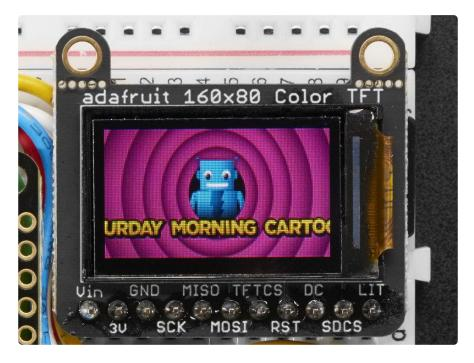
To make new bitmaps, make sure they are less than 160 by 80 pixels and save them in 24-bit BMP format! They must be in 24-bit format, even if they are not 24-bit color as that is the easiest format for the Arduino. You can rotate images using the setRotat ion() procedure
