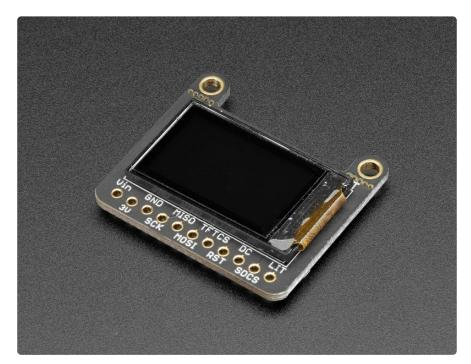
The display uses 4-wire SPI to communicate and has its own pixel-addressable frame buffer, it can be used with every kind of microcontroller. Even a very small one with low memory and few pins available!
