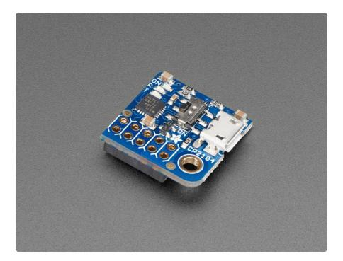
Here's another super handy add-on for your Raspberry Pi computer, perfect for 'headless' setups! The <a href="PiUART">PiUART</a> (https://adafru.it/zib) adds a MicroUSB to serial connection so you can use any serial port software to connect to the Pi's console. It plugs in and is fast and easy to add whenever you need to connect to your Pi. Two LEDs connect to RX and TX on the serial converter chip so you get blinking whenever data is sent or received.
