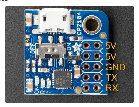
We only use the 'right' strip of the dual header but to make it more mechanically stable we have a dual header to plug into.
