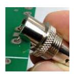
V-Bite® Edge-Mount connectors are fast and simple to install. Simply place the connector at a 45-degree angle to the PCB. Insert the PCB into the notched opening and push down onto the connector to seat it firmly in place.
