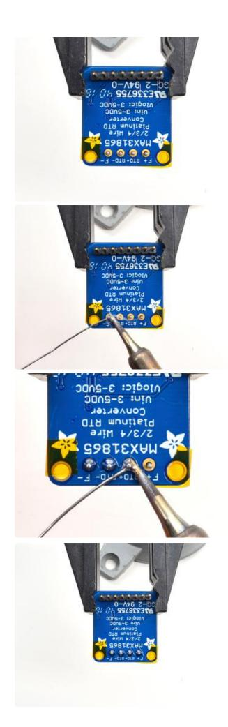
Solder in both pins of each terminal block. You can remove the tape when done.
