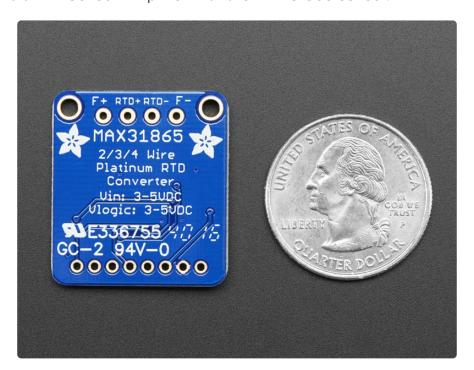
We've carried various MAXIM thermocouple amplifiers and they're great - but thermocouples don't have the best accuracy or precision, for when the readings must be as good as can be. The MAX31865 handles all of your RTD needs, and can even compensate 3 or 4 wire RTDs for better accuracy. Connect to it with any microcontroller over SPI and read out the resistance ratio from the internal ADC. We
