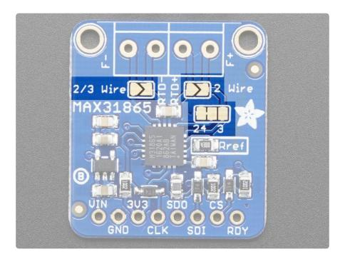
By default the sensor is wired up for 4-wire RTD usage but can be set up for 2 or 3 wire very easily.
