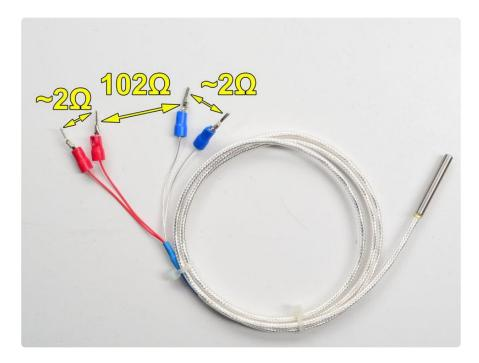
(Remember that the middle resistance - 102 or 1002  $\Omega$  - will vary with temperature, but the  $2\Omega$  wires will not) When the amp measures this sensor, it will measure the resistance between one set of red and blue wires. It will then measure the resistances between the red wires and blue wires. Then divide those resistances by half - since there's two wires and we just want the resistance of one wire. The final result is 102 - 1 - 1 =  $100\Omega$
