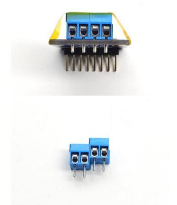
Make sure the open parts of the terminals face outwards so you can easily connect wires
