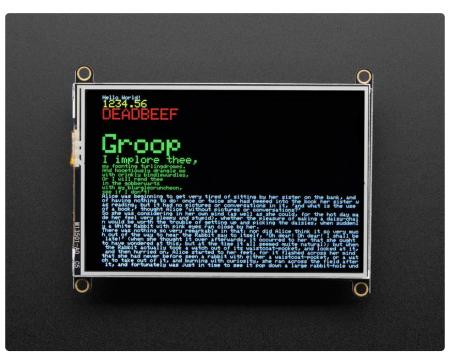
The TFT FeatherWing is basically a combination of our <u>3.5" TFT Breakout</u> (https://adafru.it/dRb) with the <u>STMPE610 resistive touch-screen breakout attached</u> (http://adafru.it/1571).
