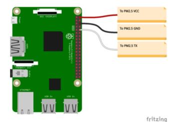
Sensor VCC to Pi 5V Sensor GND to Pi GND Sensor TX to Pi RX
