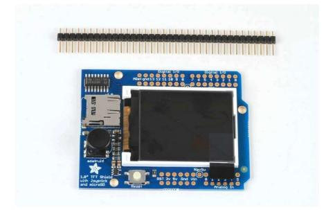
The shield comes with all surface mount parts pre-soldered. All that remains is to install the headers!
