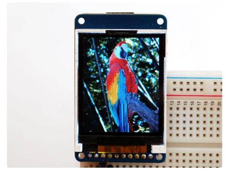
In this example, we'll show how to display a 128x160 pixel full color bitmap from a microSD card.
