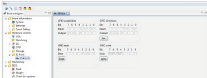
Figure 11: Configuring GPIO Pins using JIDA32/K-Station
