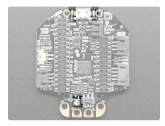
There are three LEDs - a red LED on pin D13, a CHG LED that will let you know when the battery is charging, and a NeoPixel on D8 (in Arduino) or board.NEOPIXEL (in CircuitPython)
