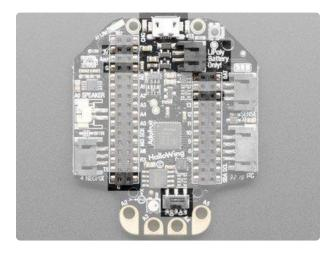
There's two ways to power your Hallowing. The best way is to plug in a 3.7/4.2V Lipoly battery into the JST 2-PH port. You can then recharge the battery over the Micro USB jack. You can also just run the board directly from Micro USB, it will automatically 'switch over' to USB power when that's plugged in
