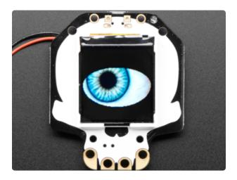
On the front is a 128x128 TFT. The TFT is connected to the SPI pins: SCK and MOSI (MISO is not connected)
