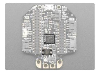
The main processor chip is the ATSAMD21G18 Cortex M0+ running at 48MHz with 3.3V logic/power. It has 256KB of FLASH + 32KB of RAM and can run Arduino or CircuitPython
