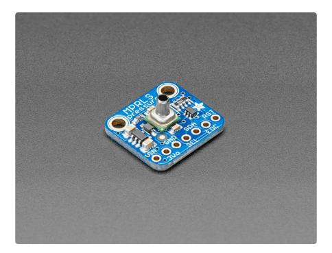
We stock a few barometric pressure sensors, great for altitude and weather measurements. This pressure sensor is special because it comes with a metal port! Unlike other pressure sensors, you can easily attach a tube to it, to measure air pressure inside a close space. In particular we think this would be a great sensor for use with making DIY assistive tech "Sip & Puff" interfaces, or measuring the pressure within a vacuum chamber or other pressurized container.
