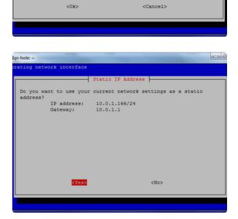
The installer will automatically try to set the dynamic IP address it got from your router to be fixed. This works well enough, if you have an advanced network set up, you can configure a custom IP address
