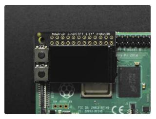
Adafruit Mini PiTFT - 135x240 Color TFT Add-on for Raspberry Pi If you're looking for the most compact li'l color display for a Raspberry Pi (most likely a https://www.adafruit.com/product/4393
