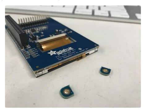
Position the PiTFT over the 2x20 GPIO connector and press downwards. Make sure the PiTFT's header is flush against the GPIO header.
