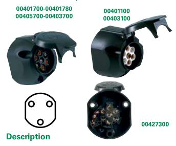
The series consists of a N (Normal) version complying to ISO 1724, which is generally used for standard applications, and a S (Supplementary) version complying to ISO 3732 to be used for additional connections. The latter can easily be recognized by its WHITE colouring and by the different order of the contacts, thus preventing an incorrect connection to the N version. Littelfuse supplies these connectors in plastic body with screw and flat contacts.
