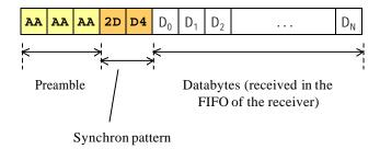
The first 3 bytes compose a 24 bit length '01' pattern to let enough time for the clock recovery of the receiver to lock. The next two bytes compose a 16 bit synchron pattern which is essential for the receiver's FIFO to find the byte synchron in the received bit stream. The synchron patters is followed by the payload. The first byte transmitted after the synchron pattern (D on the picture above) will be the first received byte in the FIFO.
