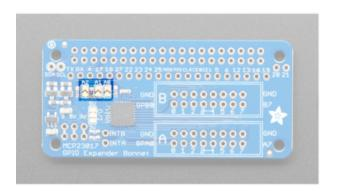
By soldering closed the address select jumpers, you can change the address from 0x20 to 0x27. This allows up to 8 bonnets for 128 total GPIO.
