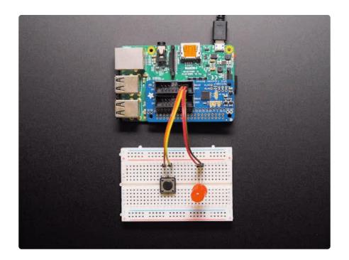
When used as an output, each pin can supply up to 20mA (current clamped) - so you can drive LEDs directly. The datasheet recommends you keep the total current draw to under 125mA for the whole chip. We set up the expander chip for 5V logic by default (the I2C is level shifted so that's 3V logic). We did that so you can drive white, blue or green LEDs that sometimes aren't too happy with 3.3V logic. Or, you can cut/ solder a jumper to change it to 3.3V logic.
