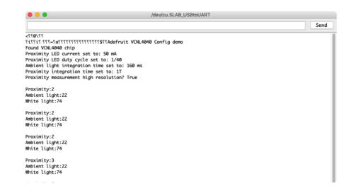
You can place your hand close to the sensor to see the proximity value change, and to see the ambient light levels change you can either cover the sensor or shine a light at it.
