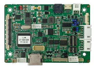
The Digital View DT-1920 LCD controller board with single HDMI input and LVDS panel connection support for general commercial and industrial applications. Compact and highly reliable this controller board incorporates advanced features such as Digital View's multi panel timing support, brightness & temperature sensors, auto-EDID setting and audio line-out.
