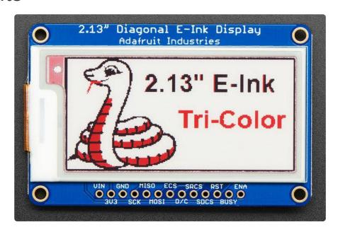
This e-Paper display uses SPI to receive image data. Since the display is SPI, it was easy to add two more SPI devices to share the bus - an SPI SRAM chip and SPI-driven SD card holder. There's quite a few pins and a variety of possible combinations for control depending on your needs
