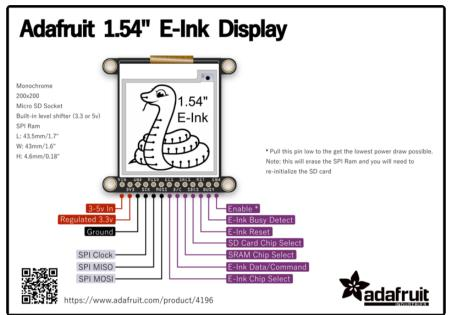
The pin outs are identical for the 1.54", 2.13" and 2.7" E-Ink display!
