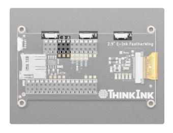
The buttons are connected to Digital Input pins. Pressing the button brings the pin low. There are no pull-up resistors connected, so you will need to enable those in software.
