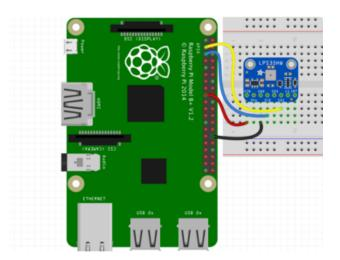
Pi 3V3 to sensor VIN Pi GND to sensor GND Pi SCL to sensor SCK Pi SDA to sensor SDI
