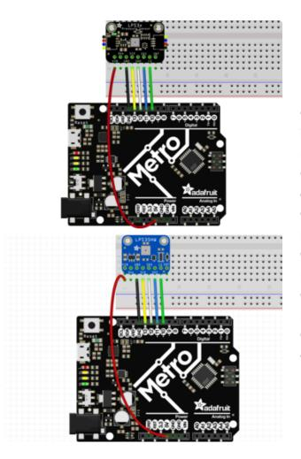
Connect Vin to the power supply, 3V or 5V is fine. Use the same voltage that the microcontroller logic is based off of Connect GND to common power/data ground Connect the SCK pin to Digital #13 but any pin can be used later Connect the SDO pin to Digital #12 but any pin can be used later Connect the SDI pin to Digital #11 but any pin can be used later Connect the CS pin Digital #10 but any pin can be used later
