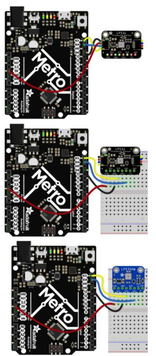
Connect board VCC (red wire) to Arduino 5V if you are running a 5V board Arduino (Uno, etc.). If your board is 3V, connect to that instead. Connect board GND (black wire) to Arduino GND Connect board SCL (yellow wire) to Arduino SCL
