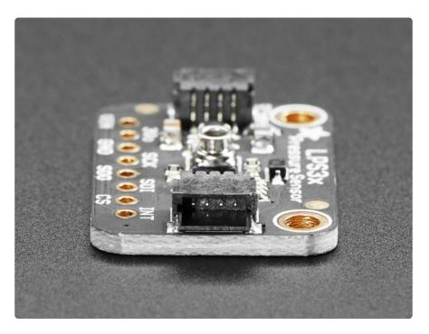
The LPS33HW also joins our growing family of boards with <u>SparkFun QUIIC</u> () compati ble <u>STEMMA QT</u> () connectors, allowing you to combine it with all sorts of <u>other</u> sensors (), and even displays (), all without needing to solder! Just plug and go/blow!
