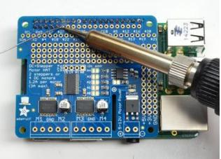
Flip the board around and solder all the connections for the other half of the 2x20 header
