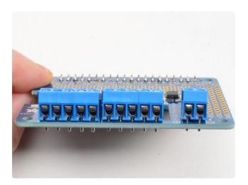
Slide the terminal blocks along the edge of the HAT, so that the 'mouth' of each block is facing out.
