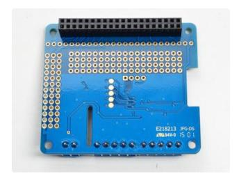
Check over your work so far, make sure each solder point is shiny, and isn't bridged or dull or cracked
