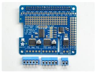
Now grab the 3.5mm-spaced terminal blocks. These will let you quickly connect up your motor and power supply using only a screw driver
