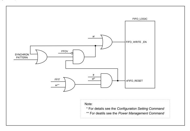
Bit 1 (ff): FIFO fill will be enabled after synchron pattern reception. The FIFO fill stops when this bit is cleared.
